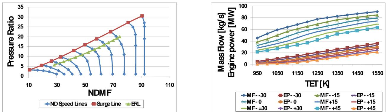
**FIGURE 2. (A)** Gas turbine performance characteristics. **(B)** Effect of changes in the ambient conditions over the Gas turbine power output and mass flow
