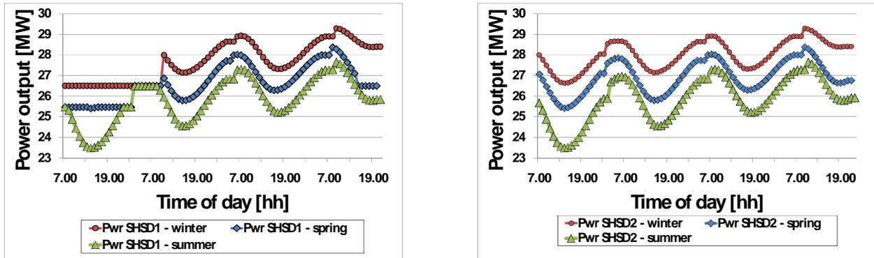
FIGURE 5. Engine power output variation in AWC with (A) 120µ and (B) 240µ of SHSD
