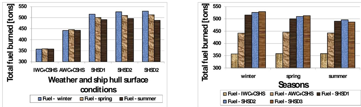
**FIGURE 12.** Comparison of the quantity of fuel burned per voyage under the effect of (A) Weather and ship hull fouling conditions. (B) Climatic conditions in winter, spring and summer seasons
