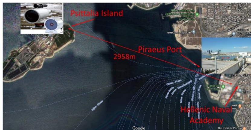
FIGURE 7. The maritime optical communications link that connects the Hellenic Naval Academy and the lighthouse on Psittalia Island and has a total length of 2958 meters [10].
