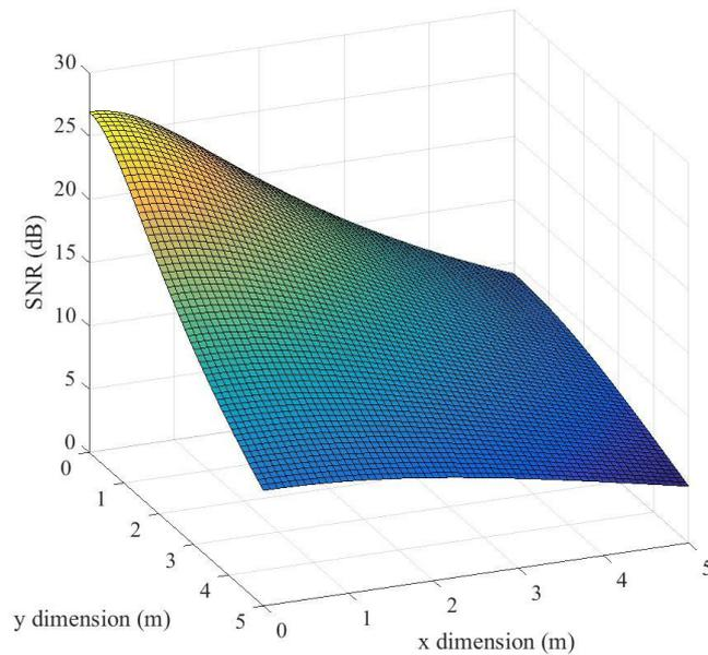
**FIGURE 6:** SNR of each LED using optical filter
