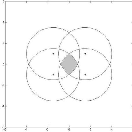
**FIGURE 3:** Overlapping Area of 4 LED lamps
