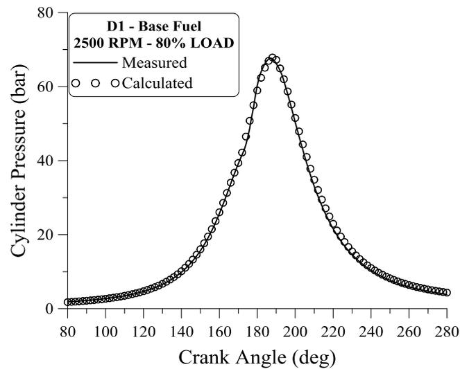
**FIGURE 3. Comparison of theoretical and experimental values of cylinder pressure of “Lister LV1” engine at 2500 rpm and at 80% of full load**
