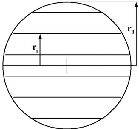
**FIGURE 2. Fuel jet distribution into radial zones [14,20]**
