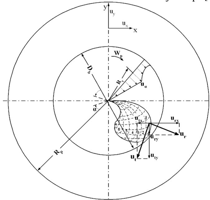
**FIGURE 1. Schematic view of the swirled air flow field and one of the fuel jets on a plane perpendicular to the cylinder axis [14,19,20]**
