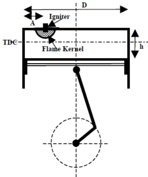
**FIGURE 1.** Schematic diagram of the flame kernel formation.
