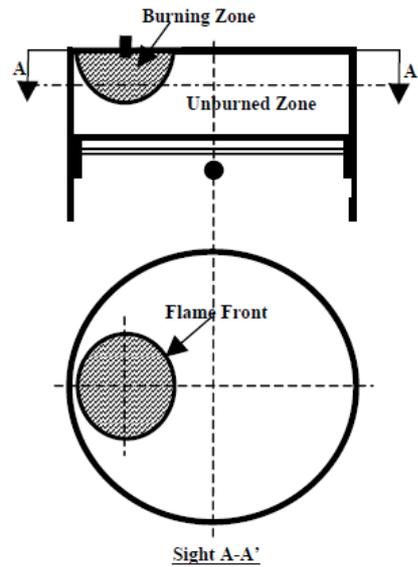
**FIGURE 2.** Two-zone thermodynamic model of combustion process.
