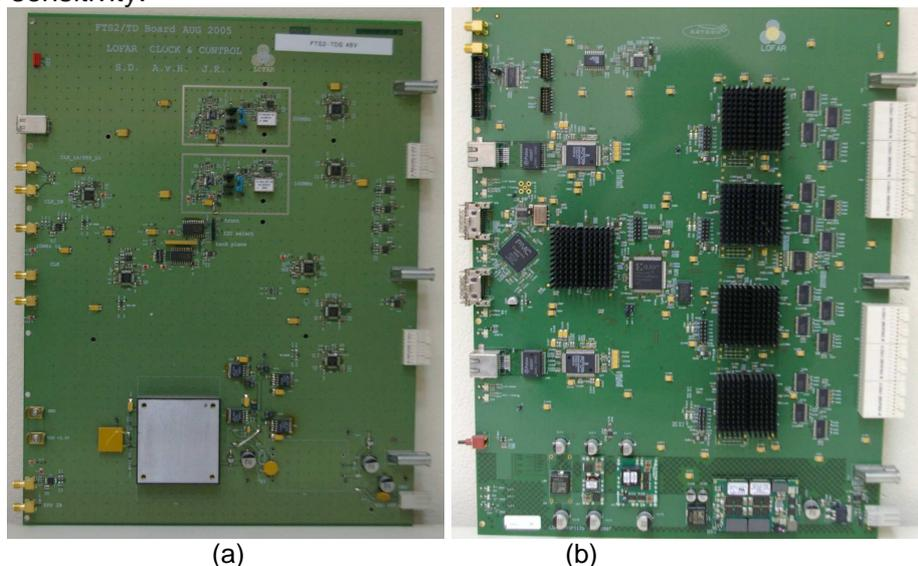
**FIGURE 4.** (a) The Time Distribution Board (TDS) and (b) The Remote Station Processing (RSP) board
