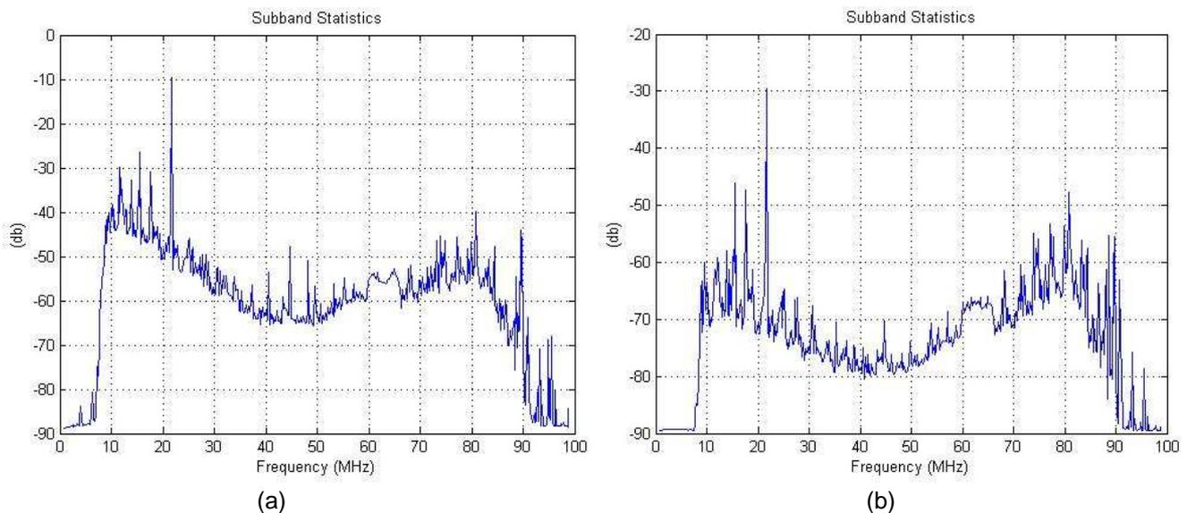
**FIGURE 6.** (a) Left Panel: Offline reconstruction of a power spectrum received from the single RF antenna during an online data taking phase, (b) Right Panel: Offline reconstruction for Y-polarity and for the same data set
