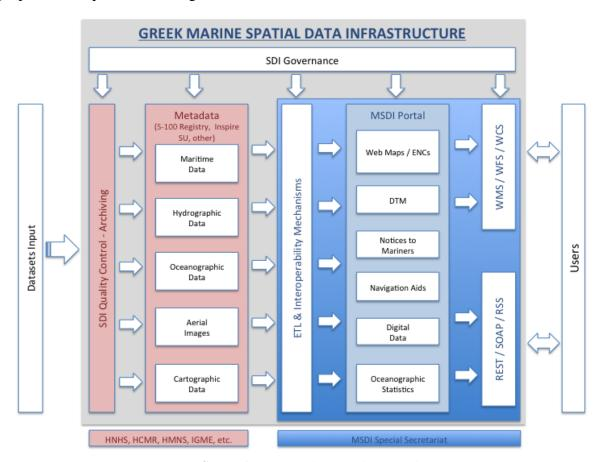
FIGURE 6. MSDI Logical Architecture Diagram
