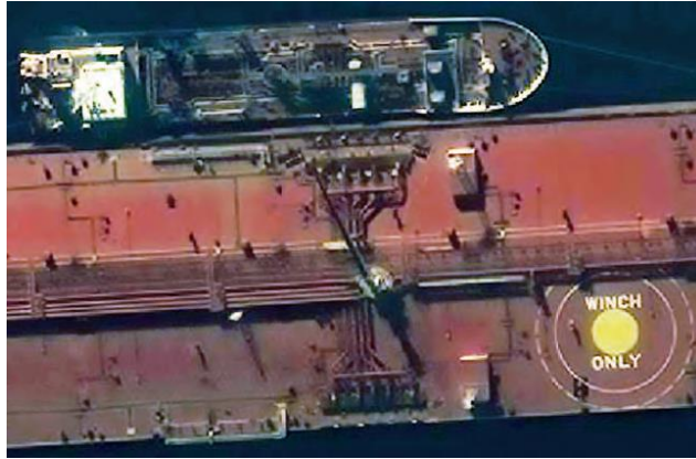
FIGURE 6. Part of a visual satellite image with 30 cm resolution. Any feature of the ship of this size, it becomes noticeable. The original image covers an area of 50 x 50 km. From: http://copernicus.eu/main/Brochure
