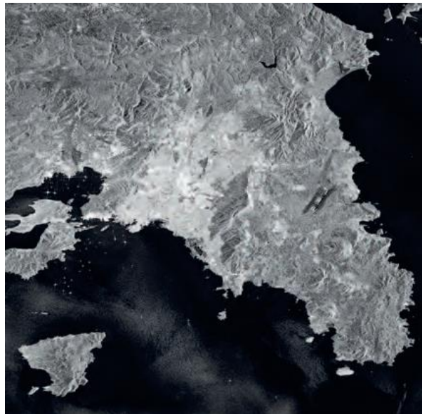
FIGURE 5. SAR satellite image section depicting Attica, with the original image covering an area of 250 x 250 km. Vessels of over 100 m in length look like bright dots at the anchorage of Salamis. From: http://copernicus.eu/main/Brochure
