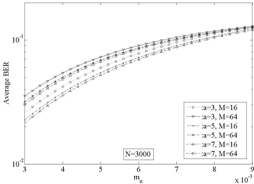
**FIGURE 2.** Average BER for the cases of strong turbulence conditions, i.e. using the K-distribution model.
